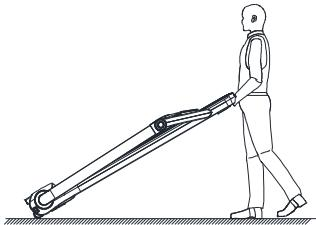
The user stands at the back of the treadmill, grasps the crossbar on the back of the treadmill with 2 hands, raises it 35°, pushes the treadmill to a suitable location and lays it flat. A safety zone of at least 2000 mm × 1000 mm should be reserved behind the mat to avoid accidents when using the mat.
