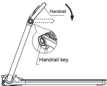
Folding the mat: While slightly lifting the mat, press the button on the side, at this time, the hand can rotate, and after rotating to a certain angle, the button can be released, and after rotating in place, it will make a "click" sound, indicating that it is locked in place.
