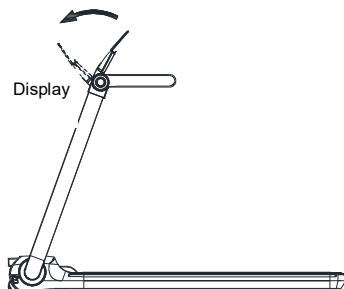
Folding the computer from the mat: Hold the computer with both hands, push the computer forward with slight force and rotate it.
